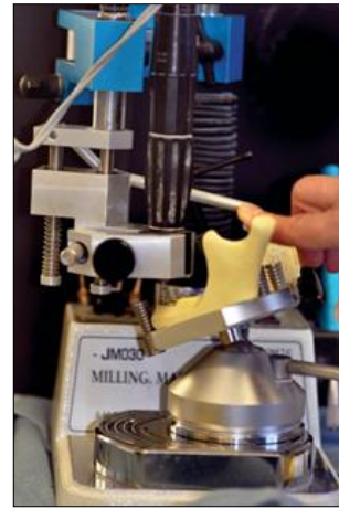
Fig 1: Placement of implant in simulated mandible before design of titanium framework bar.
