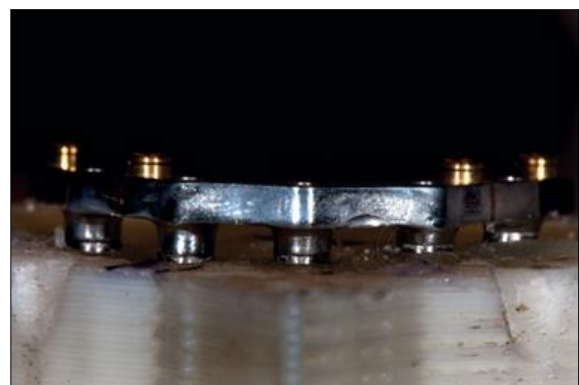
Fig 3: Milled framework attached to implants by screws (frontal view) and ready to be embedded into triangular mandibular holding device.
