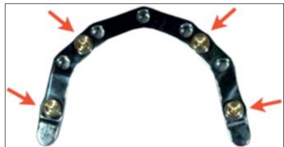
Fig 2: Fabricated milled-titanium framework with 4 locator attachments (arrows) that received loading force (test) or not (control).
